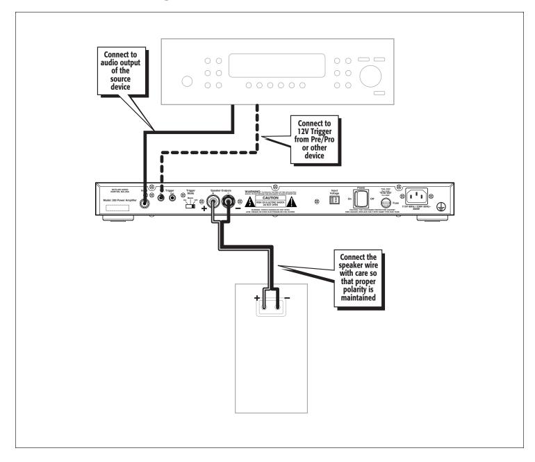
Cables with a gauge of 16 may be used for short runs of less than ten feet. We do not recommend that you use any cables with an AWG equivalent of 18 or higher due to the power loss and degradation in performance that will occur.
